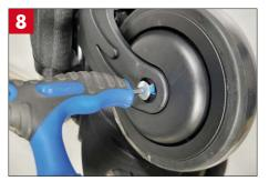
Place the male part of the screw on the other side and tighten completely.
