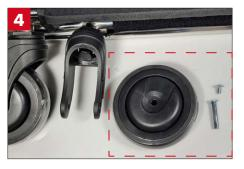
When both parts of the screw are removed, you can take OFF the wheel. All parts MUST be changed.
