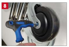
Place the male part of the screw on the other side and tighten completely.
