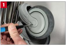
Insert the flathead screwdriver DELICATELY into the gap between the protective cover and the plastic wheel support. GENTLY action = No damage!
